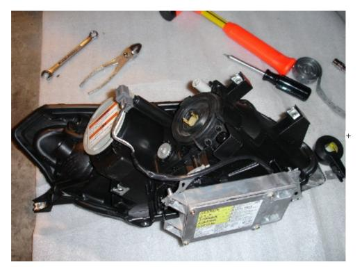
Afterwards I wrapped the parts where the housing and ballast come together with some electrical tape. Just to make sure no water or moisture would get into the housing.
