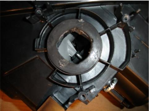
Here's what happens when you try fit the ballast into the housing.. it's just too small. After you shave the inside down you should be able to squeeze the HID ballast wiring through. It just takes a little bit of maneuvering.
