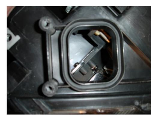
Here's the 04 housing after I cut it. I used a razor blade and a dremmel tool:
